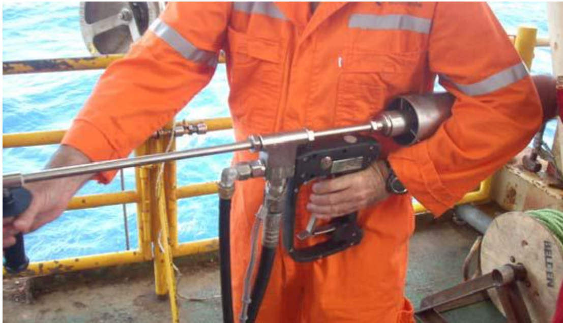
Figure 4: High pressure jetting gun lance with a protection for the retrojet venturi
